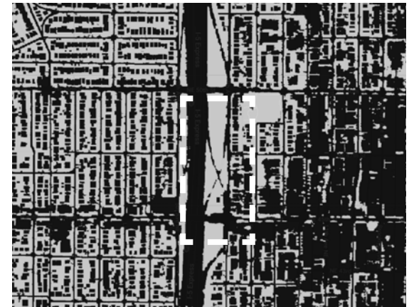
IMPERVIOUS SURFACES: Dark areas represent greater % impervious surface coverage. Image Source: Nature Conservancy
